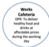
Figure 3: The starting point for drawing a Context Diagram: the System of Interest as a bubble with its Operational Requirements
